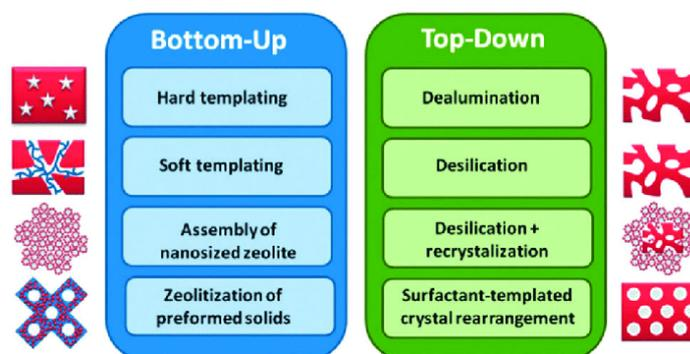
**Figure 1.** Schematic representation of different strategies of hierarchical zeolite formation [1]
