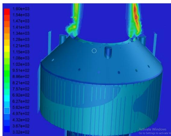
**Figure 2.** Temperature profile in the wind shield area and MP flare tip opening at operating conditions.
