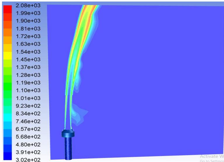
**Figure 1.** Temperature profile and flame height formed in MP flare (design conditions)
